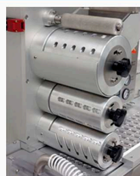
Rectification Station Feed, Rectifier & Transfer Drums
